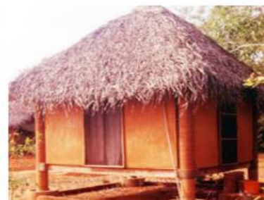
Second Legaum prototype with wattle & daub, and wooden floor
