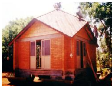
Legaum prototype with wooden shingles and interlocking CSEB
