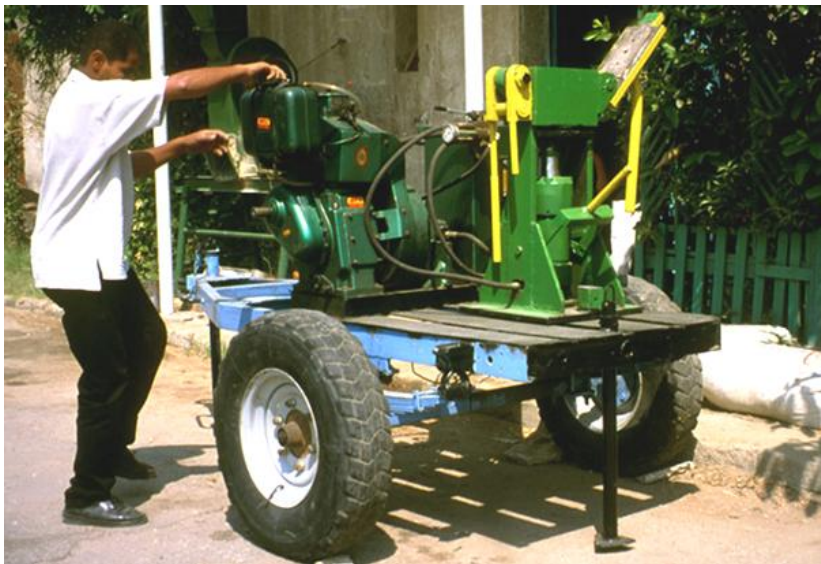
Figure 37: The machine for producing CEB designed and manufactured by EECA
