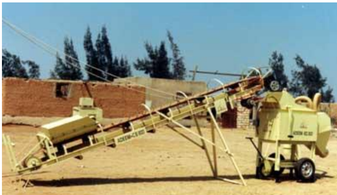
Figure 39: Mechanical production line of CEB by ADEEM. 30
