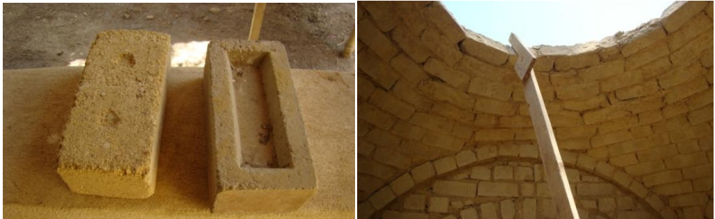
Figure 32: Lime stabilized CEB samples used in dome construction. 26
