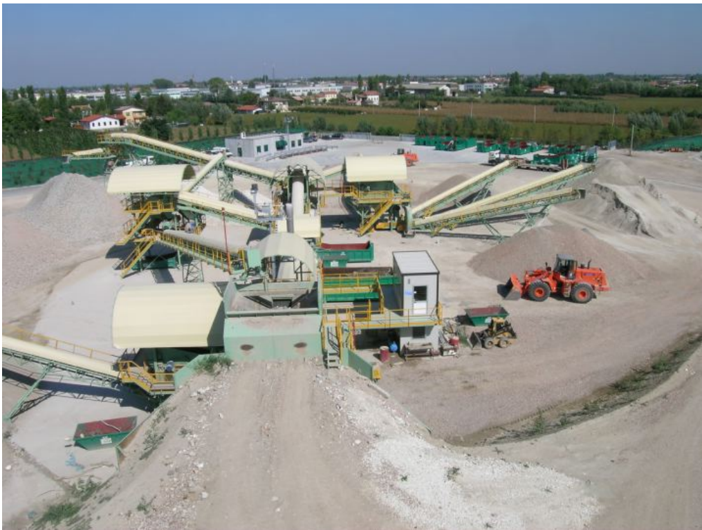
Figure 18. Typical plant for recovery and rehabilitation of C&D waste Source: Pescale Co. Italy – ROSE platform plant
