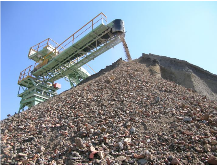
Figure 19. Stockpiling of crushed C&D debris before being sieved by size (Source: Pescale Co., ROSE platform plant)
