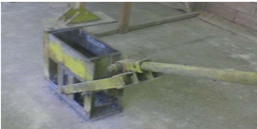
Figure 2 (a) – Production of stabilised soil bricks
