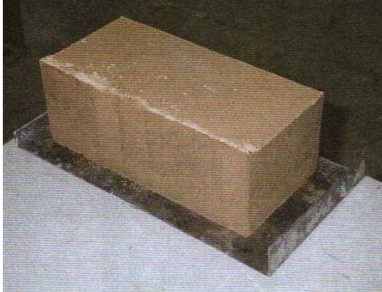
Figure 2 (C) - Stabilised-soil compacted block
