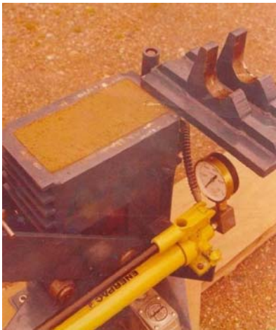
Figure 11. Stabilised soil blocks production
