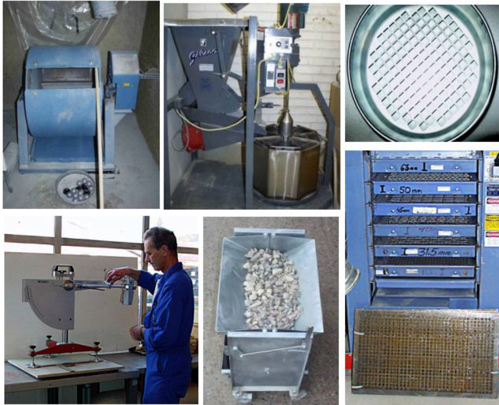
Figure 22. Tests on materials –About 30 tests are applied to qualify the aggregates obtained by crushing-sieving-sorting C&D waste. (Eng. Baratono – Italian Ministry of Infrastructures).
