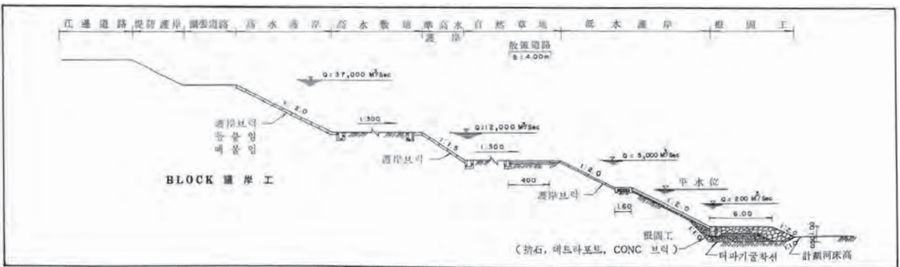
Figure 3-38. Han River Development Project, 1981-86. Typical section of embankment. Source: Seoul Metropolitan Government.
