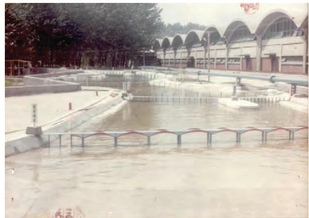
Figure 3-41. Model built to test the performance of the new hydrological infrastructure on the Han River, 1982.
