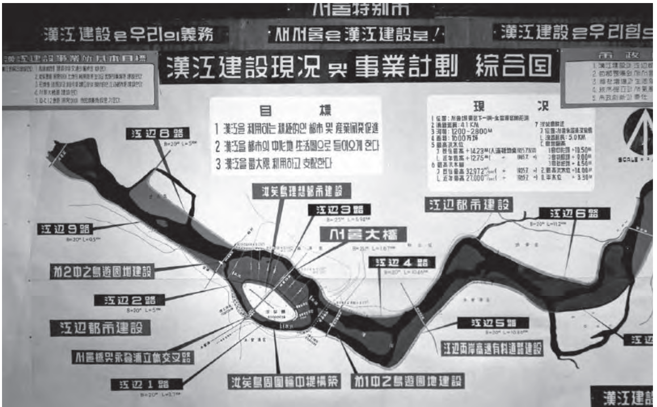
Figure 3-12. Han River Development Chart, 1968. Location of the main project areas along the river. Of special note are the tracing of the original bed of the river (in black) and the modified one (in grey), and the location of Yeouido island. Source: Seoul Museum of History (서울역사박물관).
