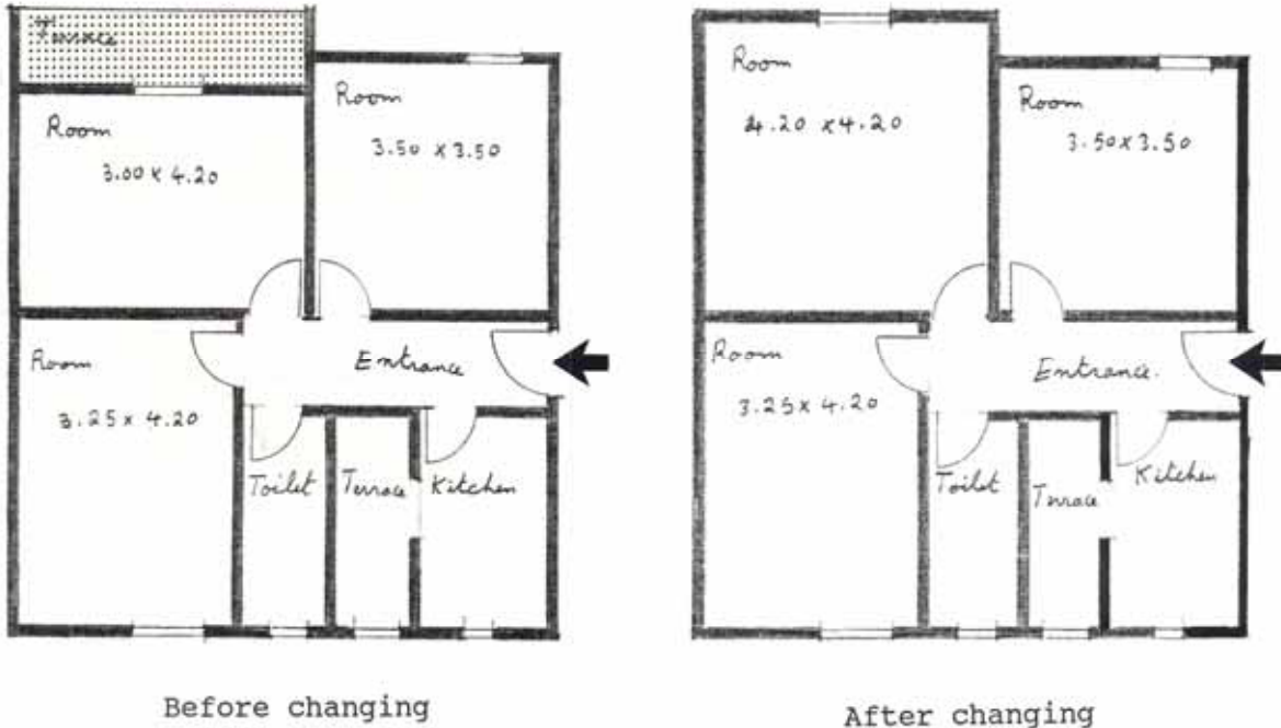
Fig. 3.20 Individual improvements in three-room apartment. Increasing the bedroom area by adding the balcony to it. Scale 1:100 (Ref. 1).
