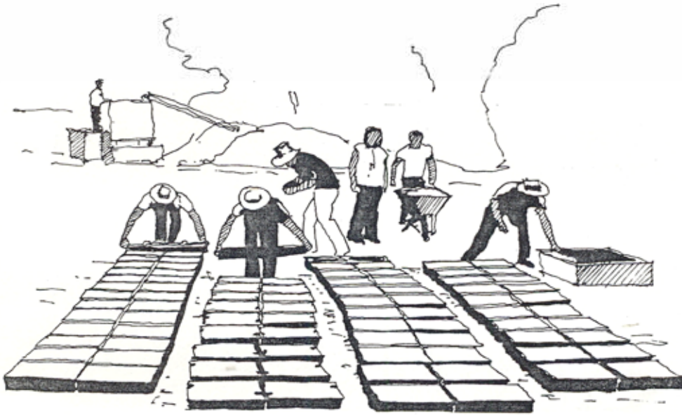
Fig. 4.19 Semi-mechanized production of adobe blocks (Ref. 20).
