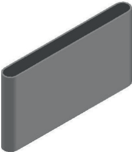
FIGURE 9: Concrete wall form constructed using CC procedure and filled with concrete.
