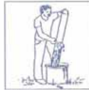
Paint them with wood preservative
