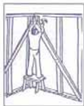
Nail corner braces
