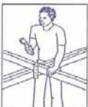
Fasten joists to Bearers with straps
