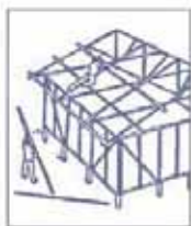
Nail purlins in place
