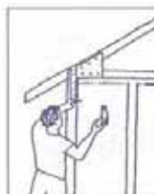
Fasten truss to wall with straps
