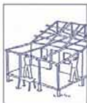
Set rafters at veranda
