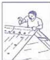
Put nail in each ridge of tin sheet
