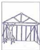
Put truss on wall
