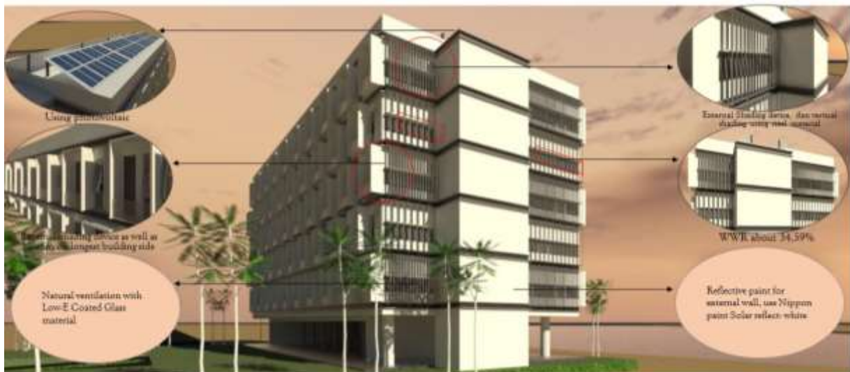
Figure 2. Visualization of a passive design concept
