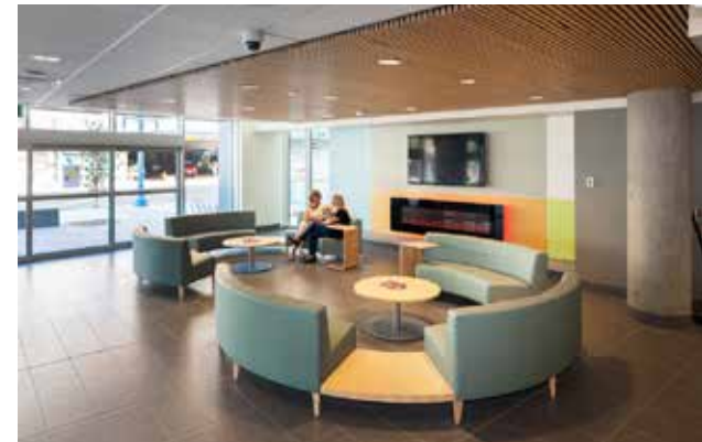
Generally speaking, neutrally coloured resilient flooring, without excessive patterning, is preferred for flooring in public areas.
