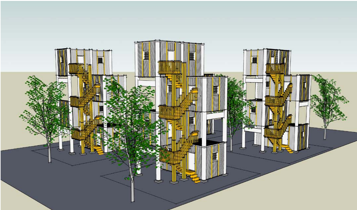
Figure 4.11 A concept for low cost housing communities composed of multistory structures assembled from adjoining basic units stacked perpendicularly up to four stories. Source: Concept by Author, and created in Google SketchUp
