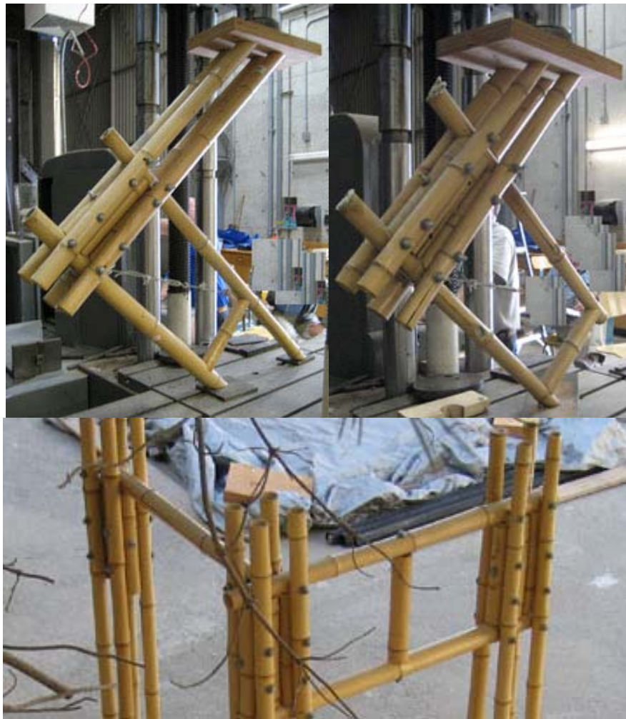
Figure 5.11 Top left: the initial test sample. Top right: modified test sample Bottom Rigid connection. Source: Photographs by Author.
