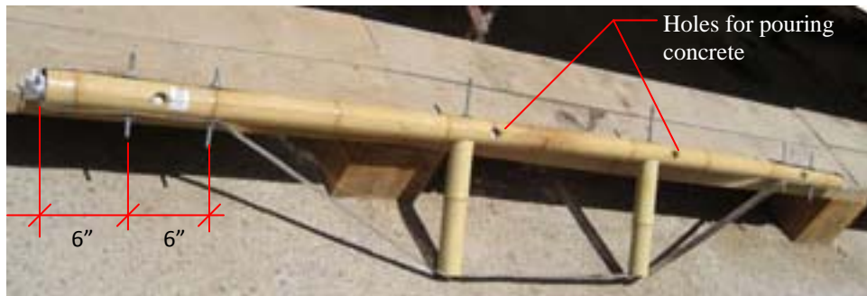
Figure 6.4 Trussed beam: Bamboo top chord, two vertical supports, 16 gauge steel strap bolted with 3/8" threaded rods. Source: Photograph by Author.
