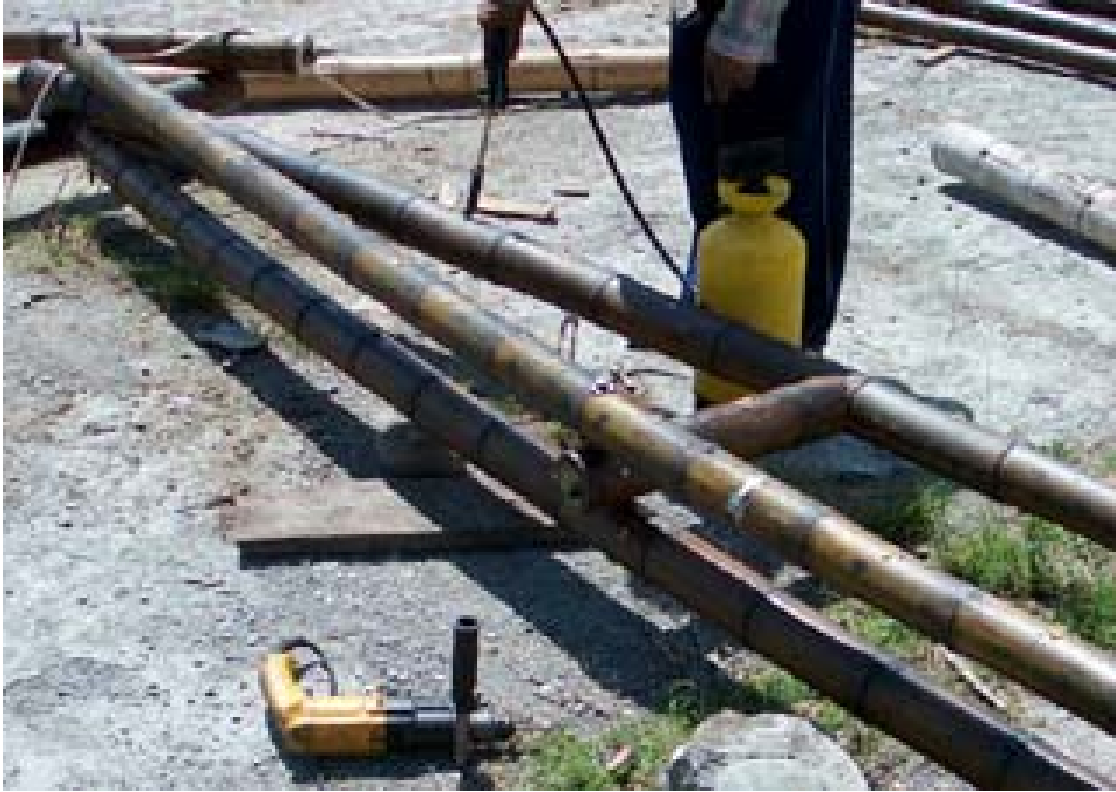
Figure 3.2 Pressure injection system used to preserve bamboo prior to application in construction. Source: http://www.mangroveactionproject.org/images/map-programs/toolkit/bamboo-treatment.jpg
