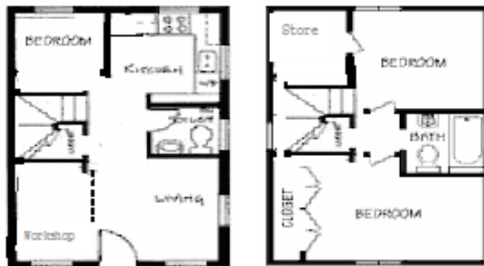
Figure 3: 34m 2 ground floor plan with additional 2 rooms on the second floor to be added as and when need arises.
