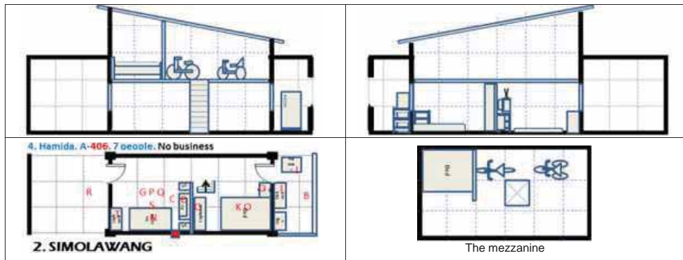
Figure 8- 17: Advantages of units located on top floor in terms of mezzanine construction
