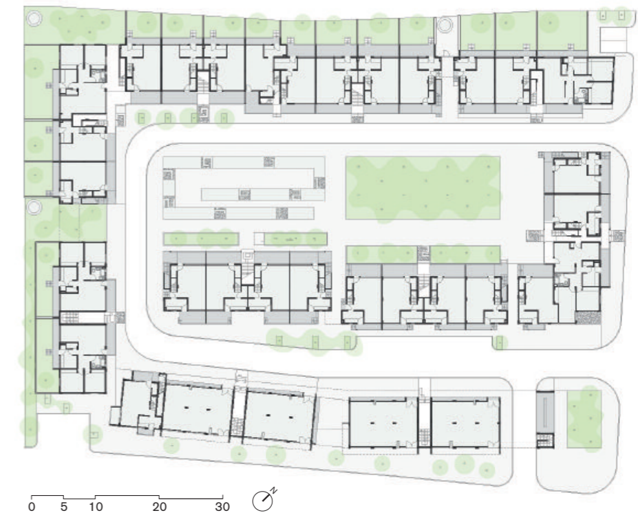
Self-wrap and permeability — Fragmented by passages, the linear building winds-in on itself acts as a porous complex of edifices rather than an introvert urban block. The gaps used for public circulation allow access to the courtyard and an internal road adds variety within to the massing.
