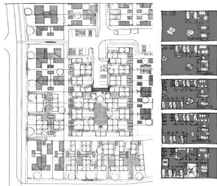
Rooms for rent — Mastering the failings of Kariobangi's and Dandora's uncompromising functionalism and negative articulation of public space, MMI conceived a sophisticated plot layout for Kayole positioning wet cores and rooms to permit the coexistence of family rooms facing a front court, and rental units arranged around a back yard.
