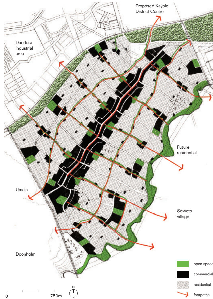
Kayole, integrated neighborhood units — At the community scale, services formed a “linear centre” along a spine road which is directly anchored to the greater urban infrastructure along which other city scale commercial functions are placed.
