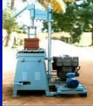
Concrete Block Machine (Sakar)
