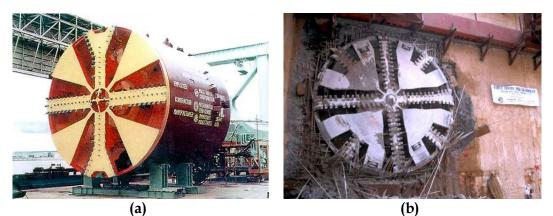
**Figure 1.** Giant Tunnel Boring Machines used in underground tunneling work in the Delhi Metro Rail Project: (a) Full view on arrival at the seaport in India, and (b) a *break-through* in hard rock strata of Delhi. (Source: *www.delhimetrorail.com*)
