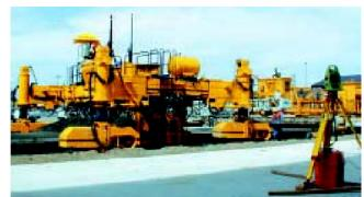
**Figure 12:** Automatically guided slip-form paving machine and on-ground monitoring systems for transferring information from ground to machine. (Source: *www.leica-geosystems.com, 2004*).
