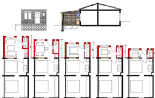
Plans of house extension options for the Roma Slum "Bangladesh" in Novi Sad Serbia. © Skat Consulting Ltd.
