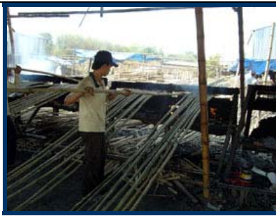
Use of fire to straighten bamboo
