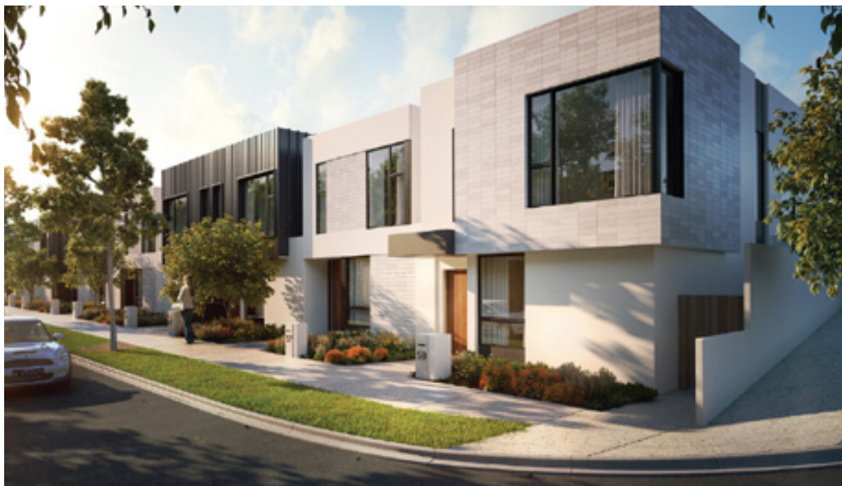
Figure 1-16 Terraces with basement parking reduces the impact of multiple driveways on the streetscape
