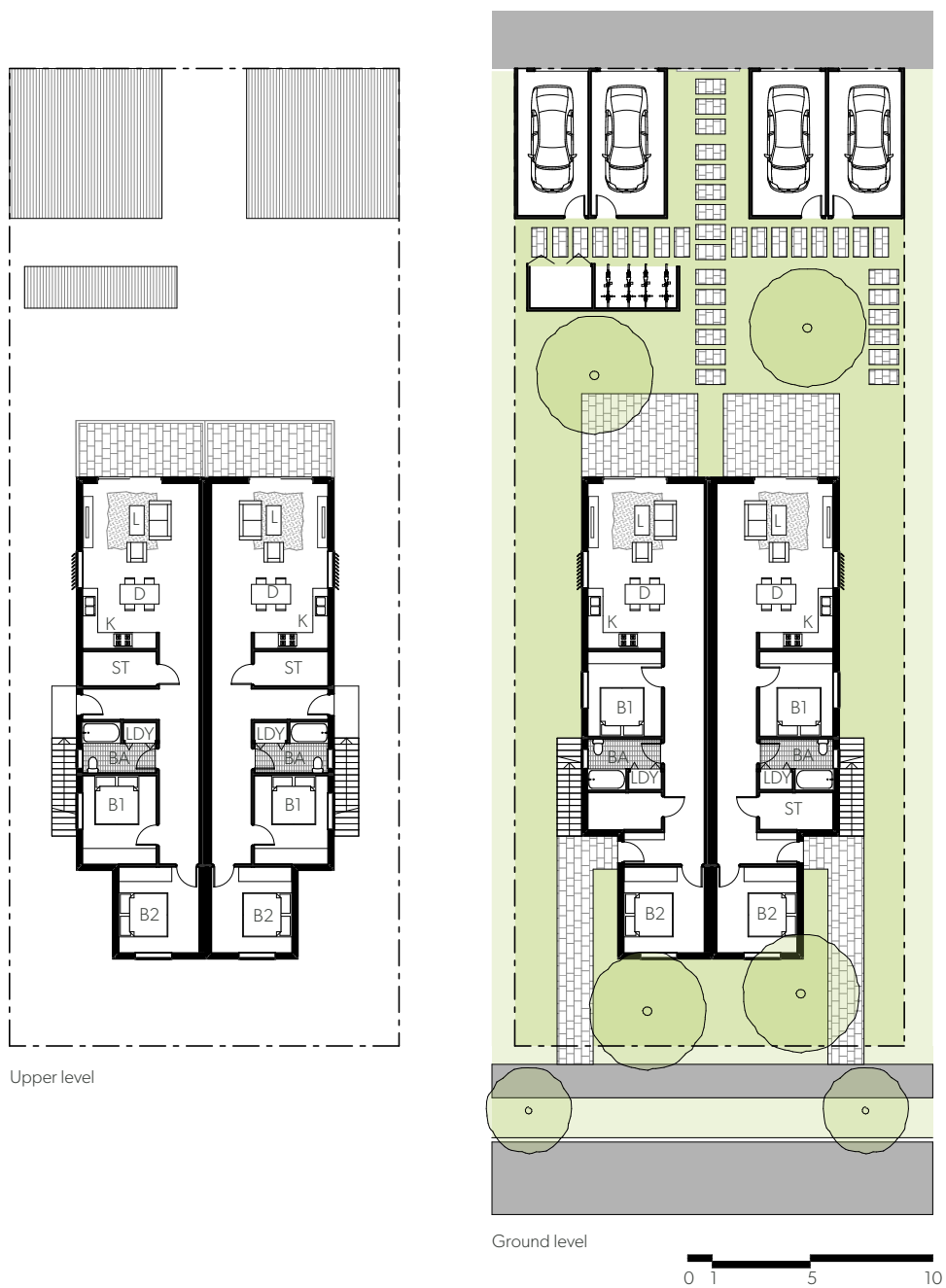
Figure 1-20 Sample plan of manor house with four dwellings and parking accessed from the rear laneway or street
