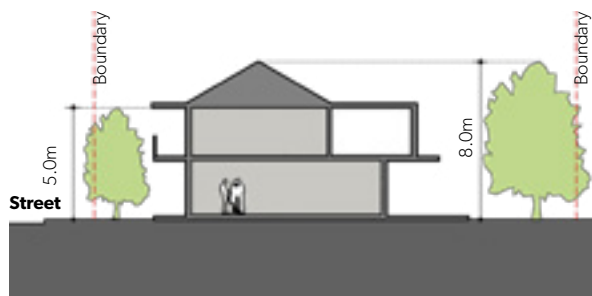
Figure 3-14 Front and rear setbacks provide opportunities for tree planting. Trees should be in scale with the development proposed
