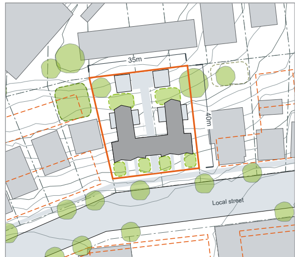
Figure 3-19 SITE SCALE: The site scale is a detailed analysis of the developments immediate context and should include the site itself, the street it addresses and surrounding properties.
