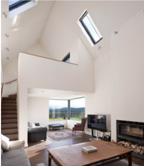
Figure 3-45 Mezzanine spaces can overlook double height spaces. The change in ceiling height and define different functions
