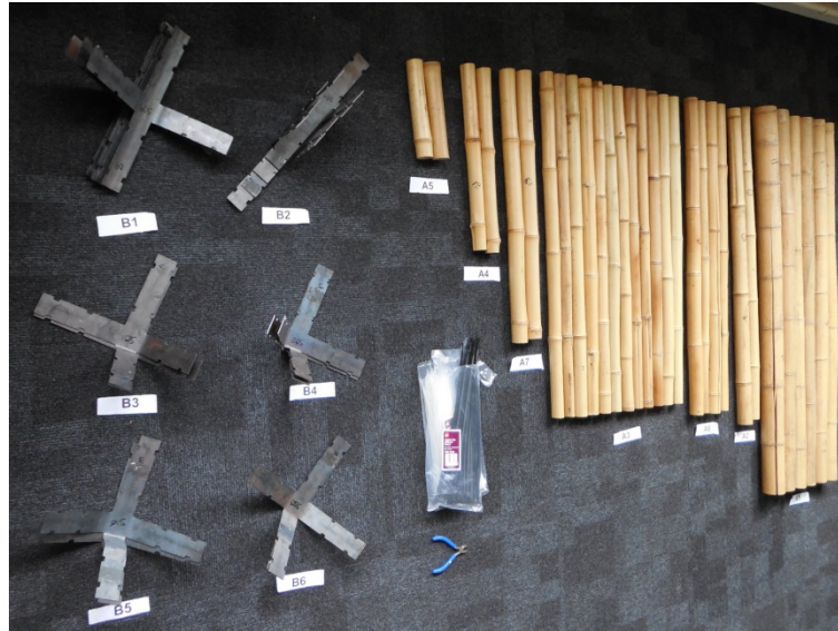
Figure 3: Parts and components as laid-out at the start of the experiments. User testing indicated that labelling was a strong feature towards feasibility of a rapid assembly
