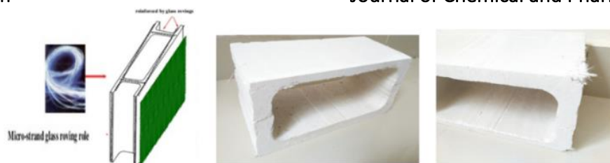
Figure.1. Rapid wall Panels reinforced with glass roving
