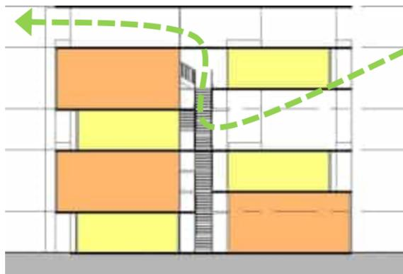
The interior alleyway, with its open aisles and stairs allows the wind inside the building, ensuring cross ventilation for all the dwellings.
