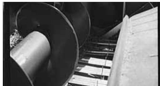
Detail of a baler showing rotating knives which cut hay into proper lengths. Photo: Pauline Ehrlich, US Library of Congress
