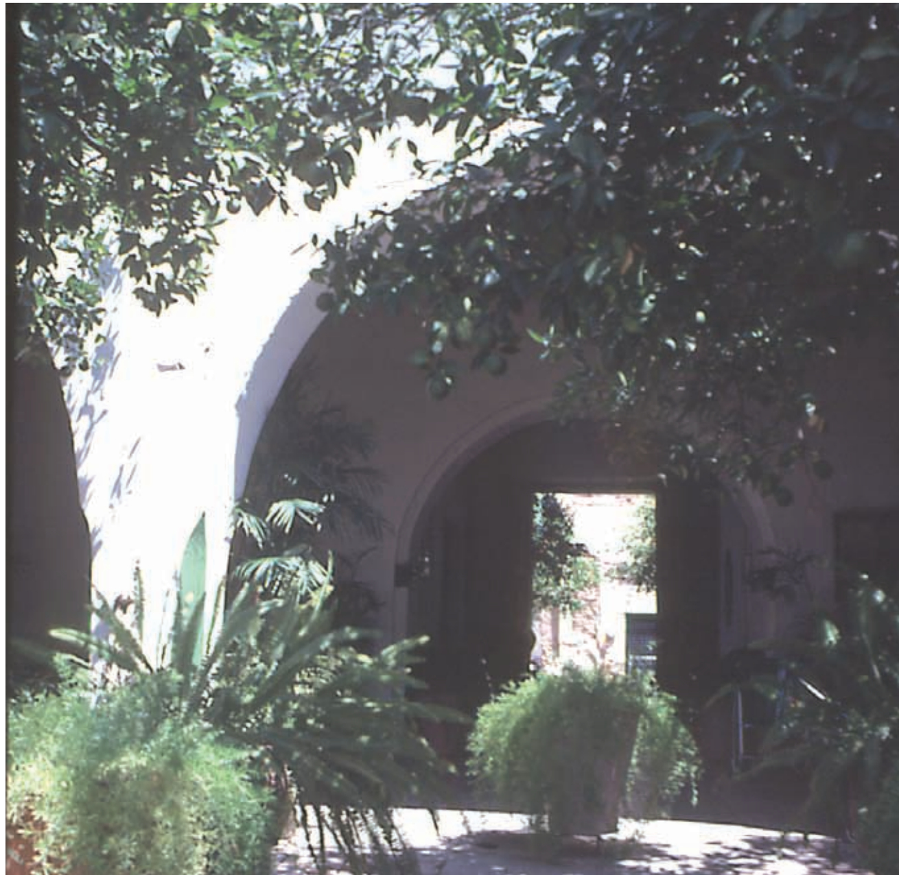
Ures, Sonora, The plant-filled patio in a traditional house cools by evaporation. Photo: B. Vint
