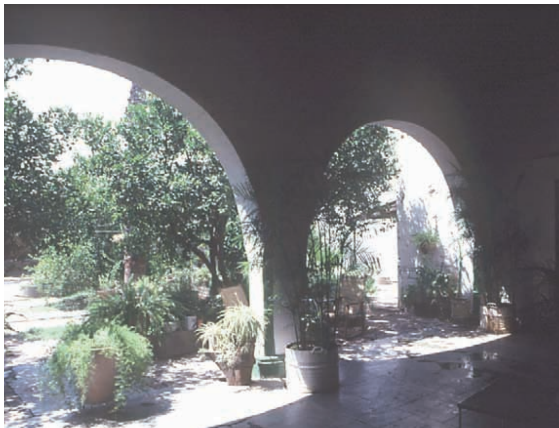
Corredor and patio of house in Ures. The corredor provides a connection between the two sides of the house, and the patio captures a small piece of the exterior, transforming it with plants and shade into a cool micro climate. Photo: B. Vint
