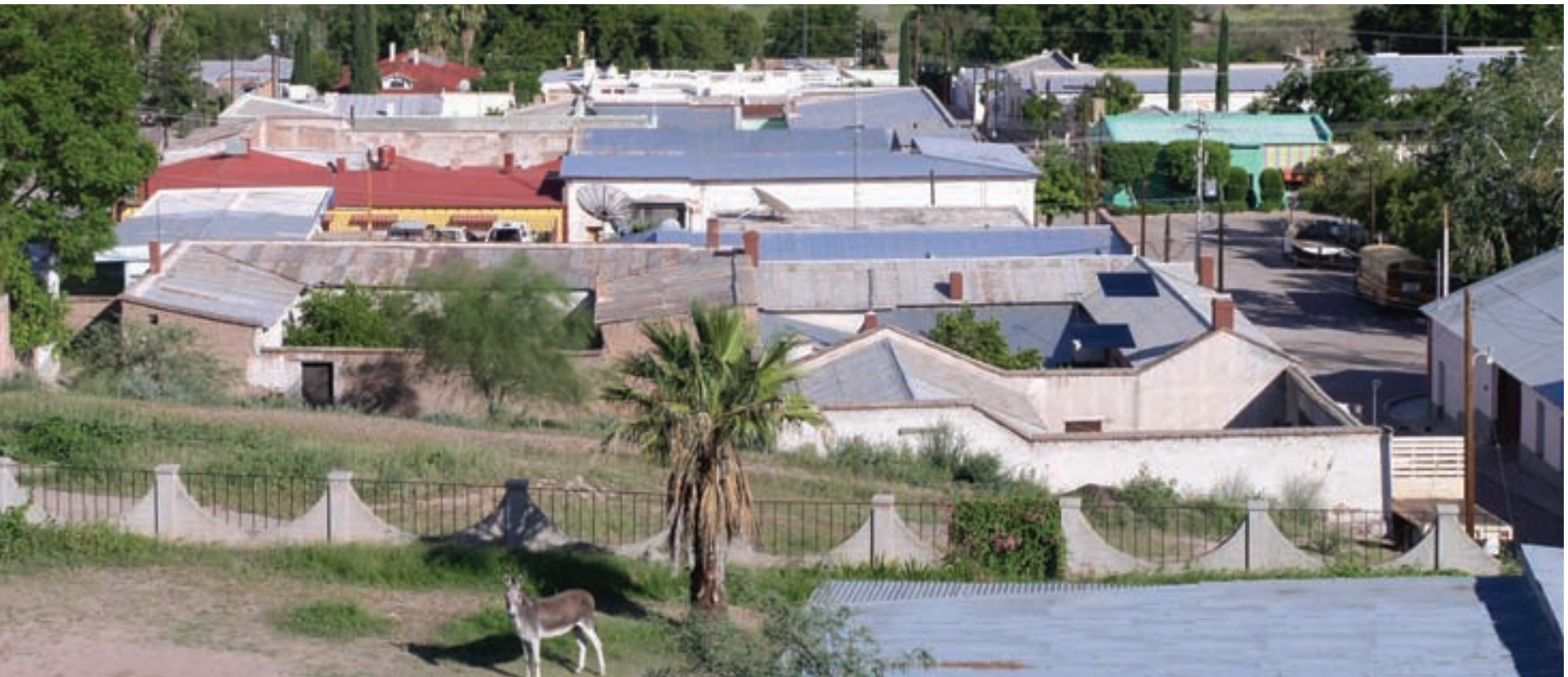
U-shaped house at center of photo is a classical Latin design. Each room opens to a central patio for privacy, fresh air and light. The courtyard is the heart of the house. Grouping of volumes creates private patios within each dwelling. Photo: B. Vint
