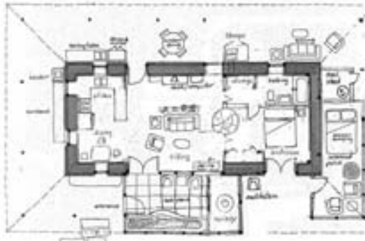
Plan of the Roberts house, planned for maximum use of limited space. The southern "Sun Room" acts as a passive solar collector. Illustration: Wayne Bingham
