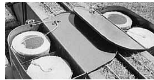
Detail of bailing machine. The propylene twine which binds the bales is inserted in spools. Photo: Pauline Ehrlich, US Library of Congress
