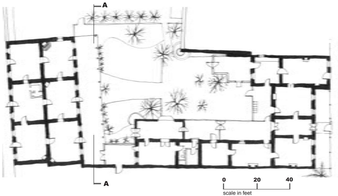
Site plan featuring large interior courtyard
