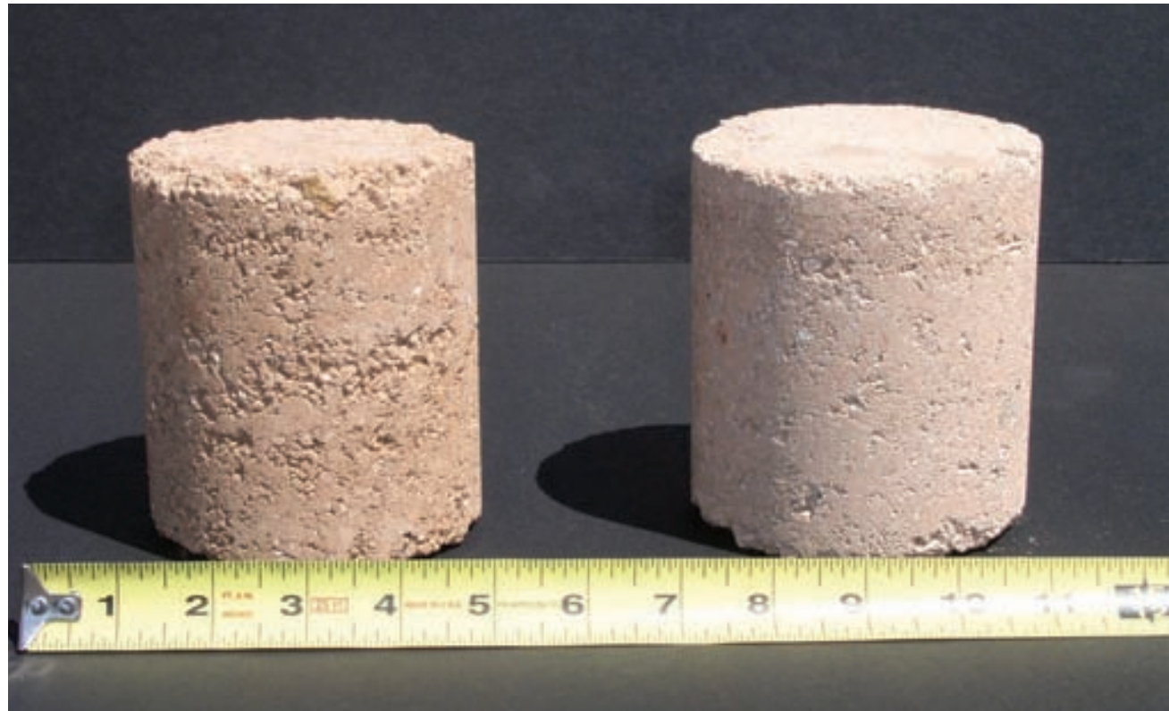
Rammed Earth test cylinders. One loaded to failure dry. One loaded to failure wet. Photo: B. Vint
