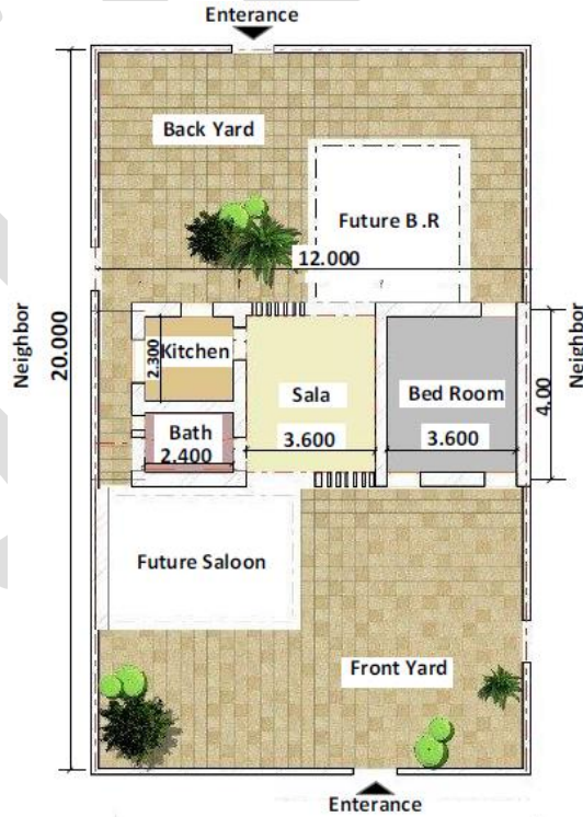
Figure (8) plan of the core unit - Al Iskan Project. Source: Ministry of Physical Planning archives
