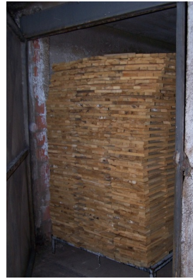
(d) Drying the wood in furnace to decrease the humid level of the wood dried in the open air
