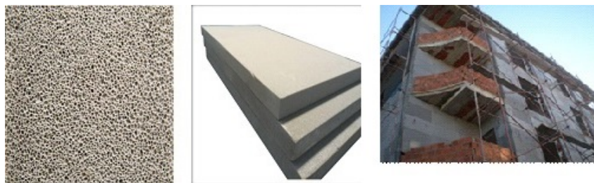
Fig. 8. Building components with wasted ceramic contained and its application.
