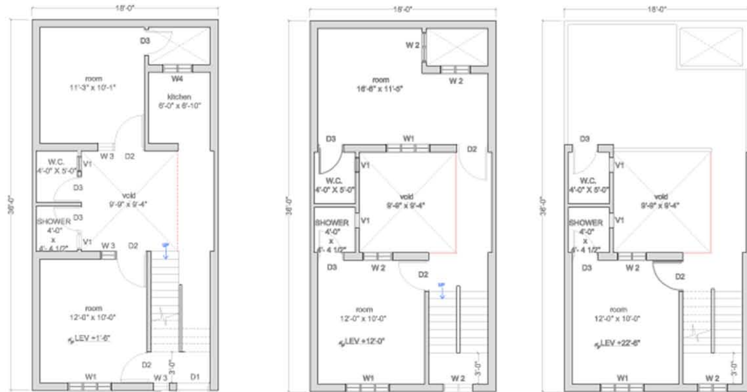
Ground Floor - 59.4sq.yds (49.7sq.m) First Floor - 55.6 sq.yd (46.5sq.m) Second Floor - 22.7sq.yds (19 sq.m) (B) PLOT SIZE: 18' X 36' - 72 sq.yds (60.5 sq.m) BUILT-UP AREA PER CAPITA: 11.5 sq.yds (9.6 sq.m)
