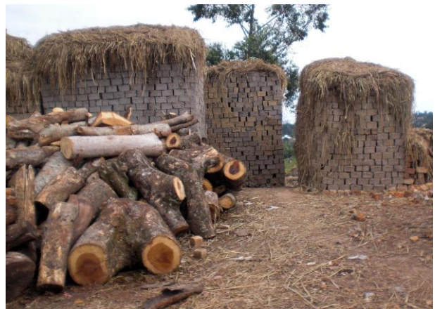
Image 4: Wood fuel at kilns at an average of 9 tonnes per burning, where 45% of the bricks might not bake in case of Rain or unexpected Night breeze.
