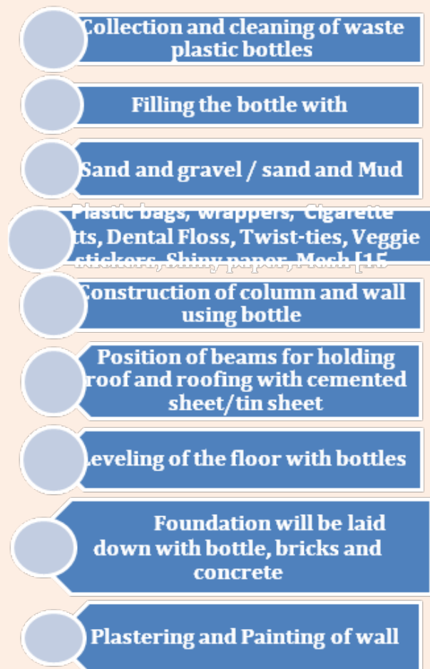
Figure 6: Methodology for construction of plastic bottle House.
