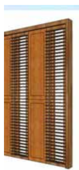
Optimized bamboo angle as a shading device
