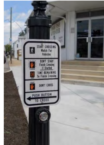
Figure 13: Accessible Pedestrian Signals in West York
