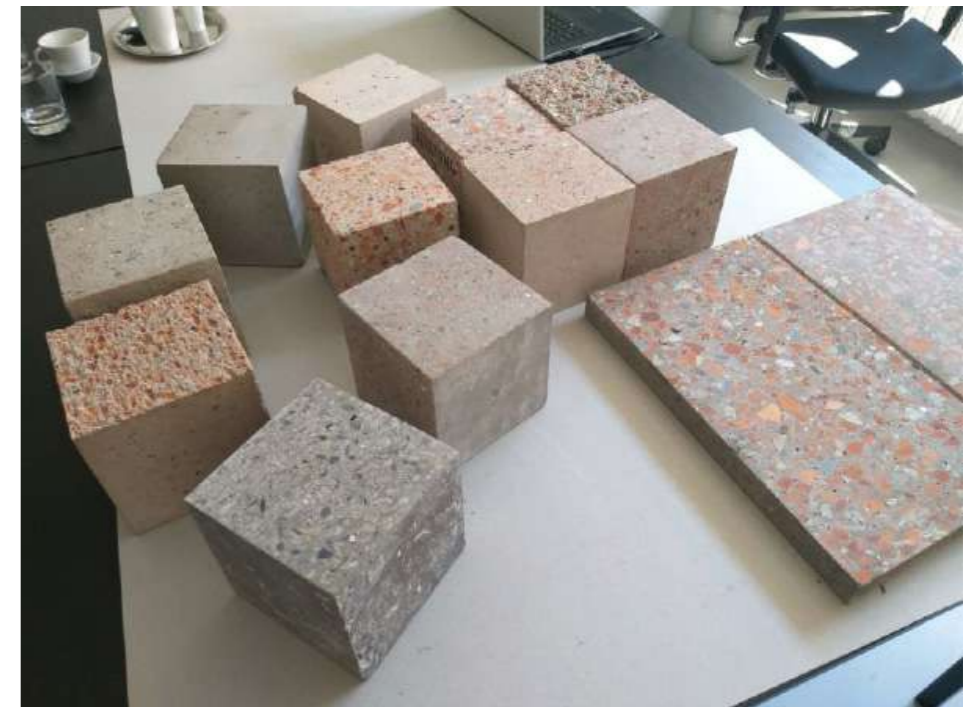
Samples of material called Rebetong, which is made from mixed recycled aggregates Source: skanska.cz
