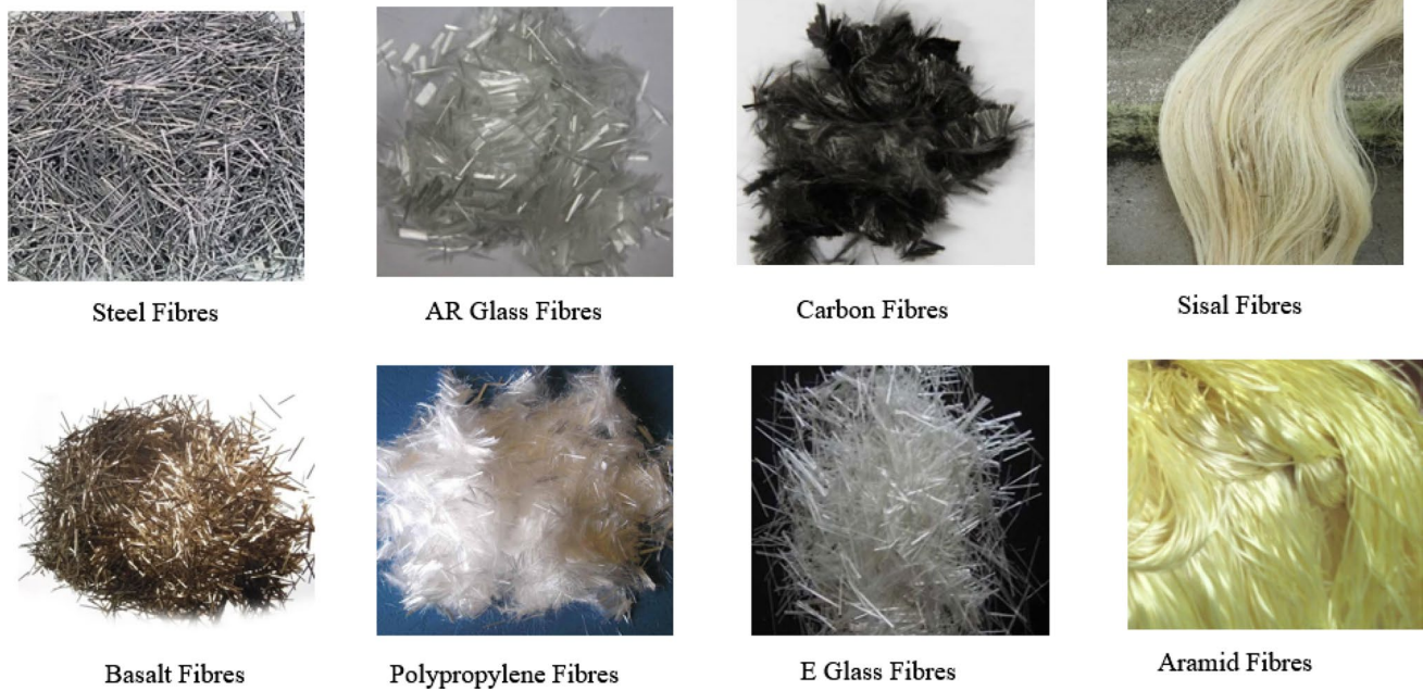
Fig. 6 Various fibers used as reinforcement in the TRC [52, 53]
