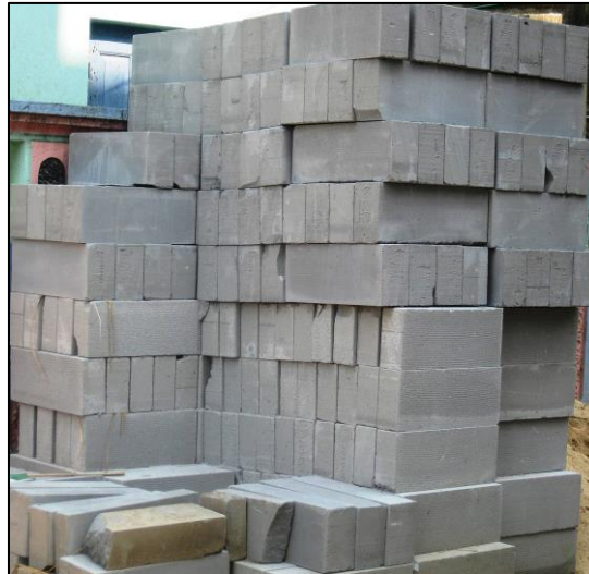
Figure 3: Solid concrete block.
