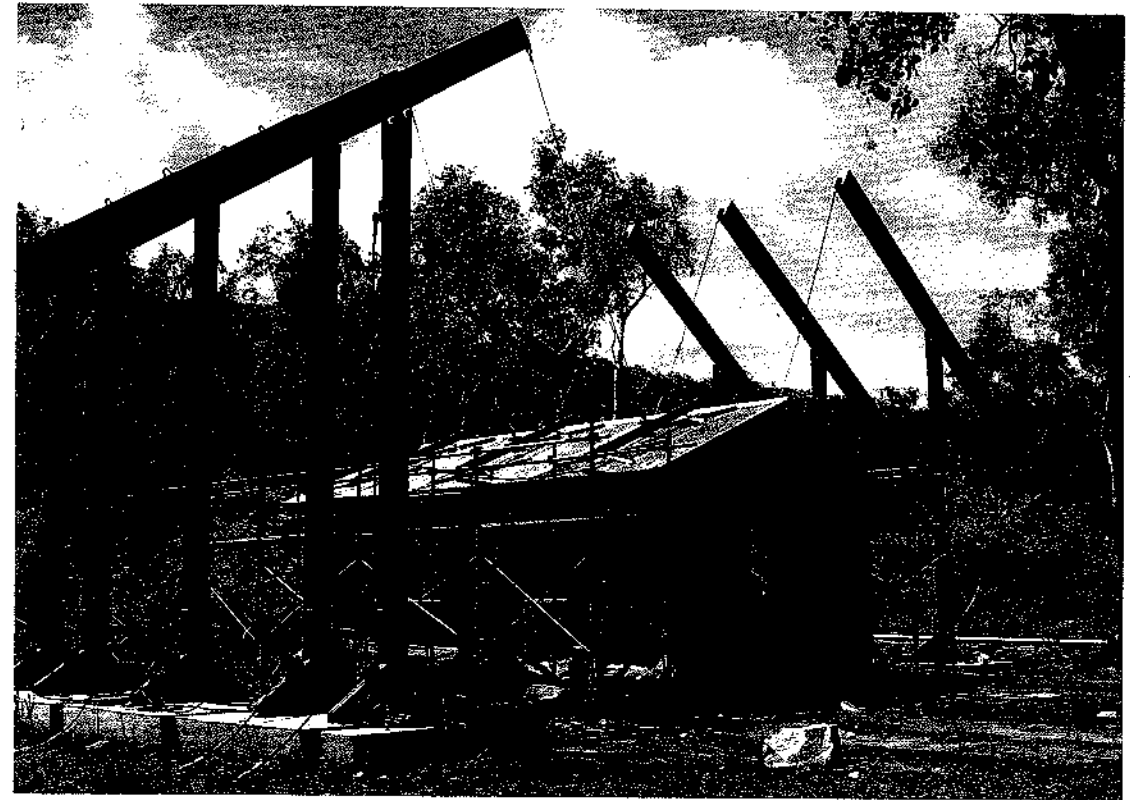
Figure 16 Cyclic loading tests on basic Tongan house
