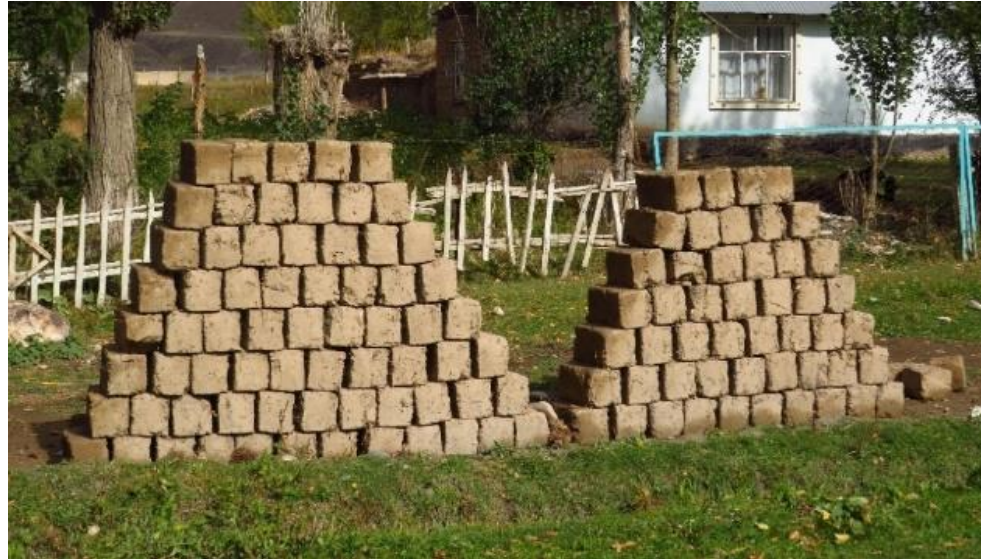
Figure 11. Clay-straw bricks being dried naturally.
