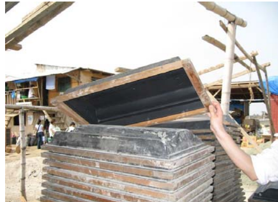
Fig. 26 Production of the roof tiles, Sanagmana, 2007-04-14
