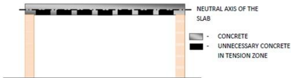
Figure5. Showing unwanted tension concrete
