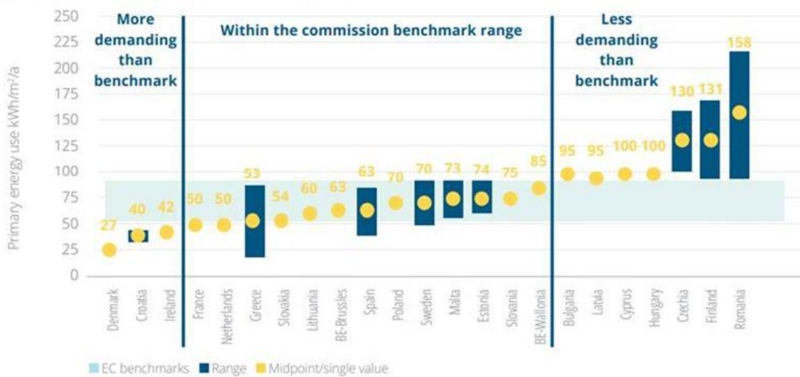
Figure 29 nZEB kWh/sqm per year values for single family homes in the EU
