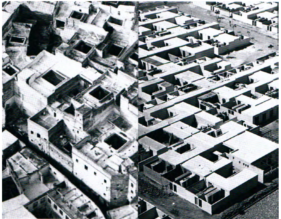
Figure 4. Re-interpretation of the traditional patio-house: Historical Morocco kasbah (left) and new urban fabric based on the Écochard Grid (right)
